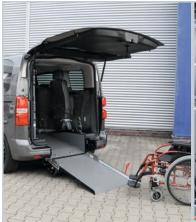
With the unfolded ramp the vehicle can be accessed comfortably with a wheelchair.
